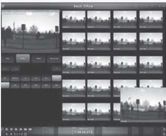
SkyPoint's Time Slicing feature automatically generates time-interval thumbnails to help identify exactly when an event occurred.
